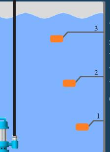
When the water level reaches the third sensor the antenna will send a signal to the nearest cellular tower, then the tower will transmit the data to our control center, which will send them to the user's cellular device.
